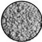
Zeolite has the ability to use a cation exchange reaction that removes other cations such as zinc, copper, lead, and ammonia from water. In the cation exchange reaction, the light metal cations in the zeolite matrix are displaced by the heavier metal cations, such as copper, in the water.
