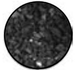
The high carbon content and porous nature of GAC accounts for its excellent ability to remove organic compounds through adsorption. Since adsorption is the physical partitioning of organic compounds to high carbon surfaces, the "activation" of the carbon (which creates GAC) endows it with an enormous surface area upon which adsorption can take place.
