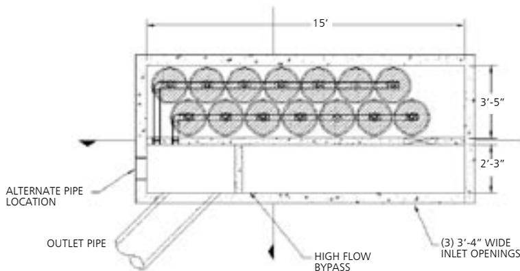
capability is based on depth of the structure. The standard bypass capacity is 15 cfs but is larger for deeper units. A traffic-bearing lid is placed underneath the median or sidewalk adjacent to the roadway.
