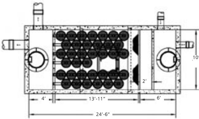
Structures range in size from a 48" manhole to CON/SPAN sections with a 24' x 10' cross section built to length. In many cases smaller structures are combined with outboard storage, such as pipe, to provide the WQv storage.
