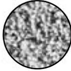
Perlite has proven to be our media of choice for sediment and oil removal. The multicellular nature of expanded perlite is the key to its excellent ability to trap sediments and adsorb oil. The coarse texture of the expanded perlite creates a bed of material with a very high porosity, which allows perlite to have the highest sediment and oil storage capacity of all of the available media options.
